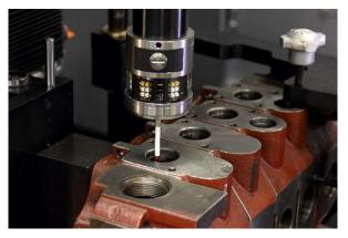
than 2,000 pounds. When a new part is loaded into the FPM-3X, the machine inspects bore locations by automatically placing a Renishaw probe into the spindle and feeding it into each bore to touch off on four sides for exact measurements. The inspection results are used to implement the required offsets and provide perfect bore positioning. The system next
