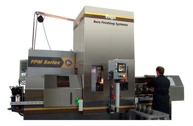
programming. These capabilities allow for the finishing of a wide spectrum of components with quick change-over. The twin-table design also lets operators load several components at once for unattended finishing.
